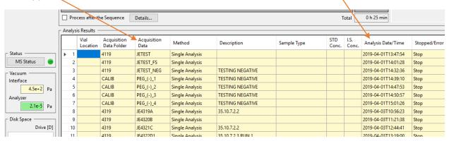
6. The time stamp can also be copied from the Data Processing window. After selecting the appropriate acquisition data file, the time stamp will be located in the 'Properties' box on the left-hand side. Highlight the time stamp and right click to copy.
