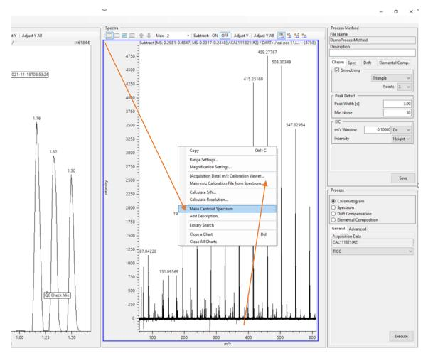
10. Then left-click on the centroided spectrum to highlight it (the software doesn't default to "choosing" the centroided spectrum, you have to click on it or the mass calibration won't work). Right-click again on the spectrum and select Make m/z Calibration File from Spectrum. A dialog window will then appear, click OK.
