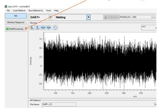
2. In the Data Processing window, select the appropriate file in the list on the left side and then right click the highlighted data (#1 is 20V, #2 is 30V, #3 is 60V, #4 is 90V) and select Open TICC.
