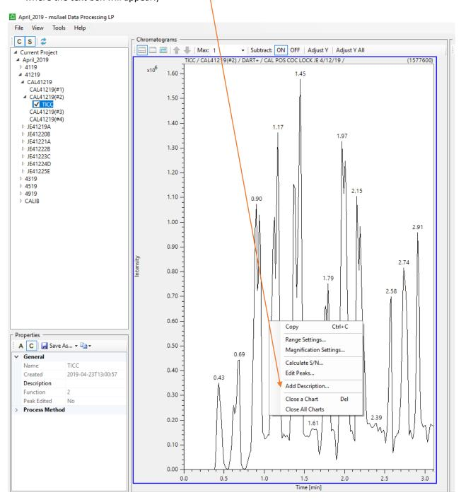
4. The TICC will not print with a time stamp so it must be added manually using the Add Description feature. The time stamp can be copied from two places. On the upper left side of the MSAxel@LP window (not Data Processing window), select Monitor/Sequence.
