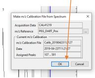
11. The m/z Calibration window will appear. The max residual (max error in MassCenter) should be less than 0.003 and the RMS residual (standard error in MassCenter) should be less than 0.001. Also, the 1-R and 1-R\* should show values with e-012 for a good calibration. The polynomial order should remain at 3. Outlying data points can be removed on the PEG600 spectrum. Left-click on the data point, then right-click and select Release. No more than two, non-adjacent data points should be removed.
